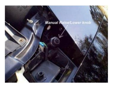
Start with the headlight in the down position. Remove the plastic (or sometimes rubber) cover over the headlight motor assembly and use the Manual Raise/Lower knob to raise the headlight to the full up position.
