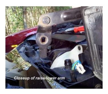
This next part is important! You now need to, while CLOSELY watching the motor shaft, rotate the raise/lower manual knob so the motor shaft turns exactly 180 degrees (or half a revolution). Once you have completed this, reattach the headlight raise lower arm. What you have just done is made it so the actual motor gear will now be in contact with the \*other\* half of the plastic gear. Sure, the teeth on the plastic gear are stripped, but they are stripped on the now unused side of the gear:)
